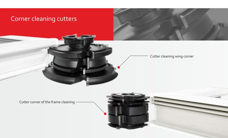
These cutters are intended for cleaning welded window corners to remove excess material. The two basic types are cutters for frames and cutters for sashes. The blades are made from carbides specially selected for milling of PVC. We use carbides from the best global suppliers only.
