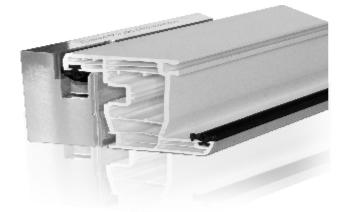
We make the support blocks from durable aluminium alloys. Support blocks for profiles with welded seals are provided with seal forming knives that are made of stainless steel of improved hardness. Upon the customer's request, we can provide the support blocks with additional knives for 0.2 mm flash forming.
